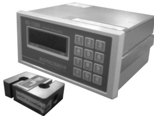
Fig. 6. A digital indicator and a load cell.
